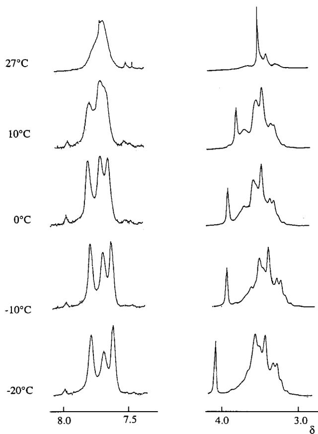
Figure 5. Partial VT  $^1\text{H}$  NMR spectra of a 1:1 mixture of **2a** and  $\text{AgSO}_3\text{CF}_3$  (acetone- $d_6$ - $\text{CDCl}_3$  3/1; 270 MHz).
