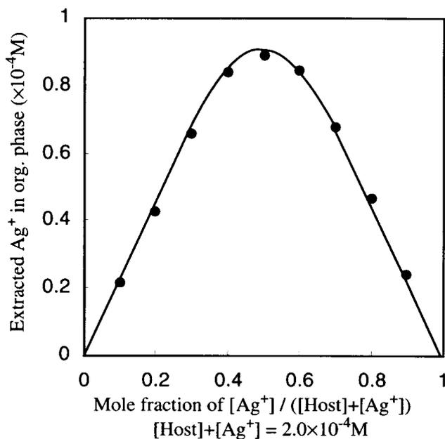
Figure 4. Job plots of the extractions of  $\text{Ag}^+$  with host **2a**.
