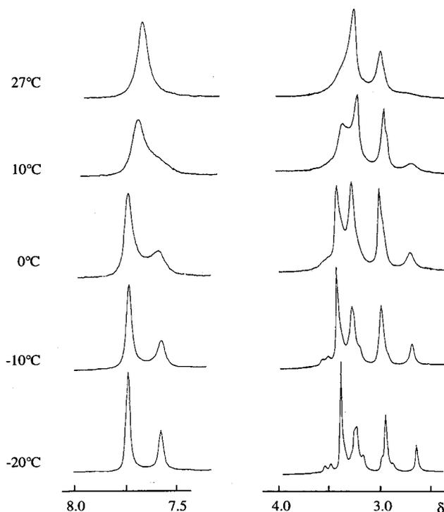
Figure 2. Dynamic  $^1\text{H}$  NMR spectra of **2a** ( $\text{CDCl}_3\text{-CS}_2$  1/3; 270 MHz).
